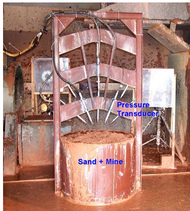
Fig. 6 A photograph of the experimental setup used in Ref 36 to study the effect of explosion of a shallow-buried mine
